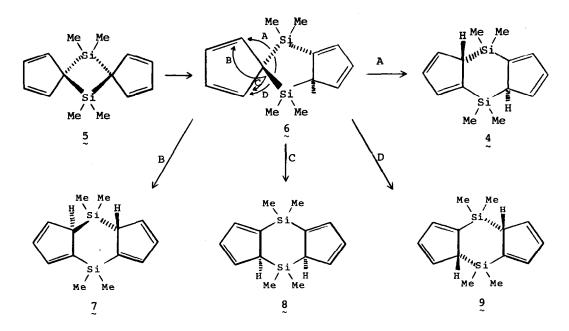
This latter result effectively eliminates the possibility that isomerization is occurring through prototropic rearrangements, since prototropic rearrangements in cyclopentadienyl silanes always occur slowly compared to the NMR time scale.<sup>9,11</sup> Thus, in solution 4 immediately established an isomeric equilibrium through a variety of facile 1,5-sigmatropic silyl migrations. The possible isomers of 4, which could interconvert by 1,5-silyl migrations, include structures 5 through 9.
